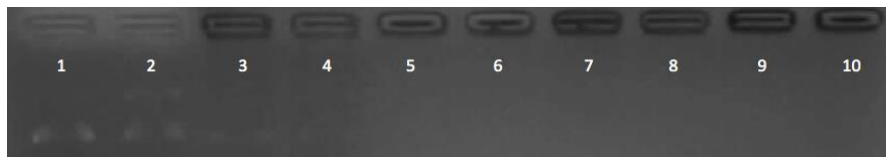
Figure 8. Gel electrophoresis diagram: Lane 1: DNA control; lane 2: DNA + H 2 O 2 ; lane 3: compound 2 + DNA; lane 4: compound 2 + DNA + H 2 O 2 ; lane 5: compound 2a +DNA; lane 6: compound 2a + DNA + H 2 O 2 ; lane 7: compound 2b + DNA; lane 8: compound 2b + DNA + H 2 O 2 ; lane 9: compound 2c + DNA; lane 10: compound 2c + DNA + H 2 O 2 .
